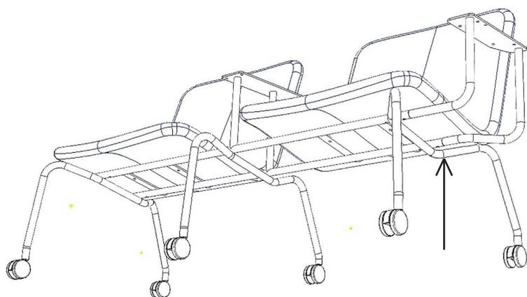
Secure them by screwing the M6x20 mm screws through the tubes into the armrest(s), 4 screws/armrest.
