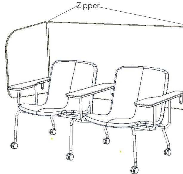
Continue assemble the side screens. Assemble the zipper in the corner and fasten the screen brackets with the M6x20 mm screws into two T-nuts underneath the armrest top and two tapered holes in the metal part. There are clearance holes in the armrest tops for these screws.
