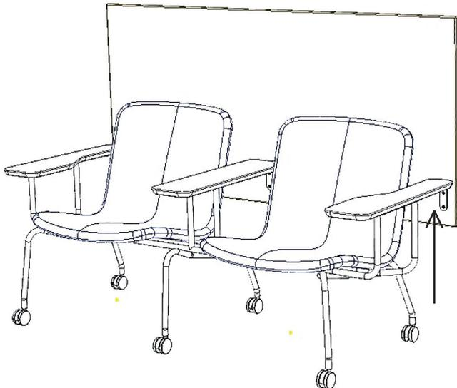
Start to assemble the back screen. Use the M6x20 mm screws into the T-nuts underneath the armrest tops.
