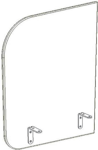
Fasten the brackets onto the screens with the countersunk M6x20 mm screws. Two brackets for the side screens and two or three for the back screen.
