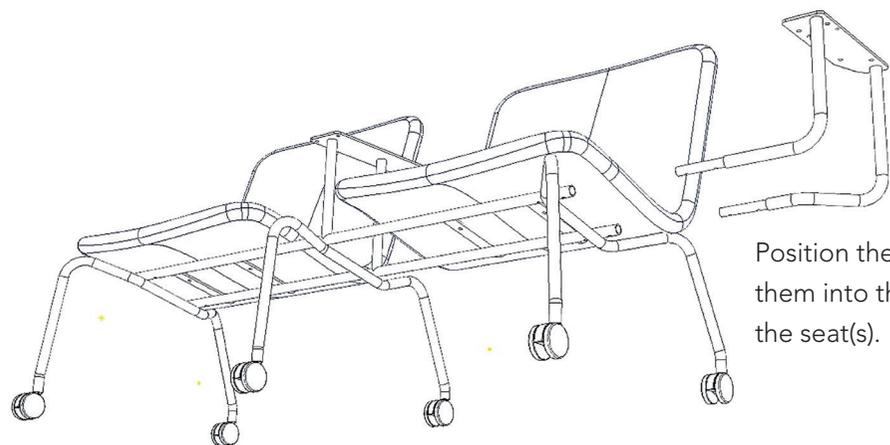
Position the armrest(s) by sliding them into the tubes underneath the seat(s).
