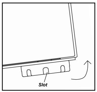
Use screwdriver in the slots to turn the foot
