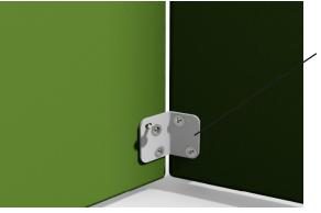
Angled bracket fittings, used in <u>inner corners</u> instead of feet. Use the oval holes to adjust the leveling.
