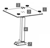
Install the Control Box (part 8) with two(2) of the ST5x16 Screws (part 5).
