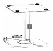
Attach the desktop to the leg (part 4) four (4) M6x10 screws (part 6). Connect the cable exiting the leg (part 4) directly into the control box (part 8). Connect the handset (part 9) cable to the control box (part 8). Connect the power cord (part 13) to the control box (part 8).
