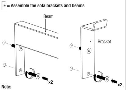
Positioned as illustrated with beam on top. Both illustrations use 2x MF6S M8x35 countersunk on each bracket/beam gable.
